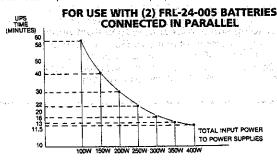
USE THESE GRAPHS TO DETERMINE HOLD-UP CAPABILITIES. POWER IS INPUT POWER OF POWER SUPPLIES.  $P_{IN} = \frac{P_{OUT}}{EFFICIENCY}$ .
