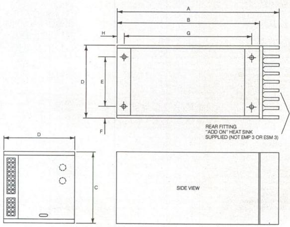
NOTE: FIXINGS ARE 8 OFF M4 THREAD—4 TOP AND 4 ON BASE OF UNITS. ALL DIMENSIONS ARE IN MILLIMETRES.
