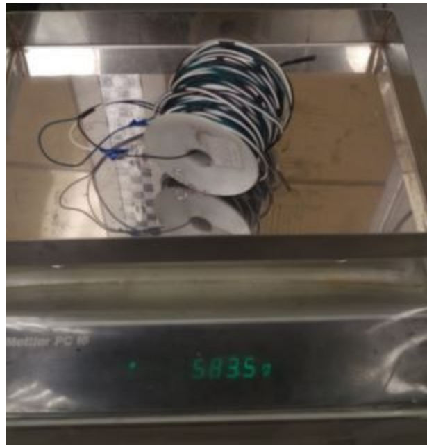
Figure 14: Completed Tether Cable on Spool (Weight = 5845 - 39 = 545 grams = 1.2 lb)
