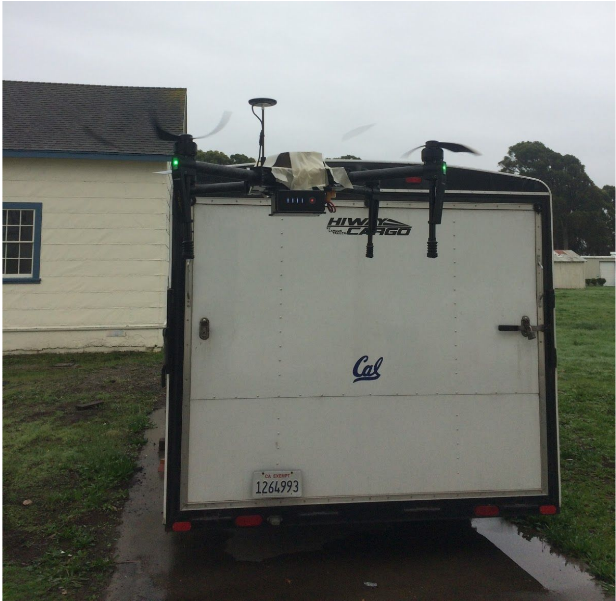
Figure 21: Payload Test - Drone carrying 5 lbs
