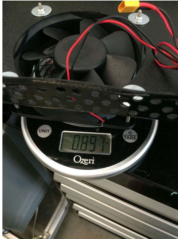
Figure 17: Final Weight of Onboard Power Supply Case (Weight = 0.9 lb)
